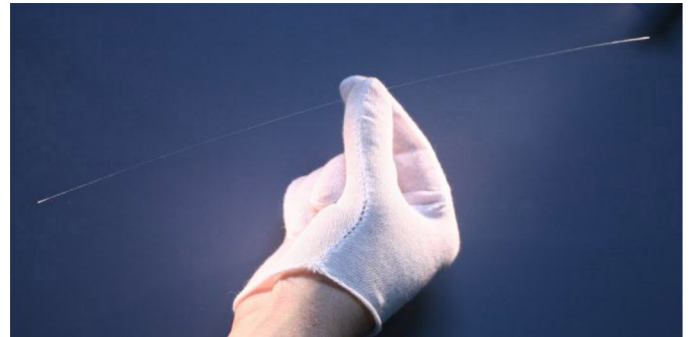
Figure 1. A doped single-crystal yttrium aluminum garnet (YAG) fiber.
