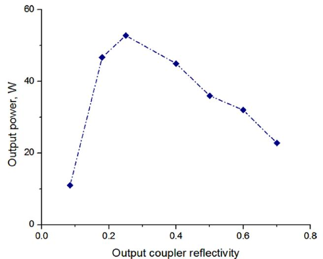
**Figure 3.** Laser output power (Q-CW) versus output coupler reflectivity measured at pump power of 91.6 W. The plot clearly indicates the optimum reflectivity as 25%. Connecting lines are only used as a guide to the eye.
