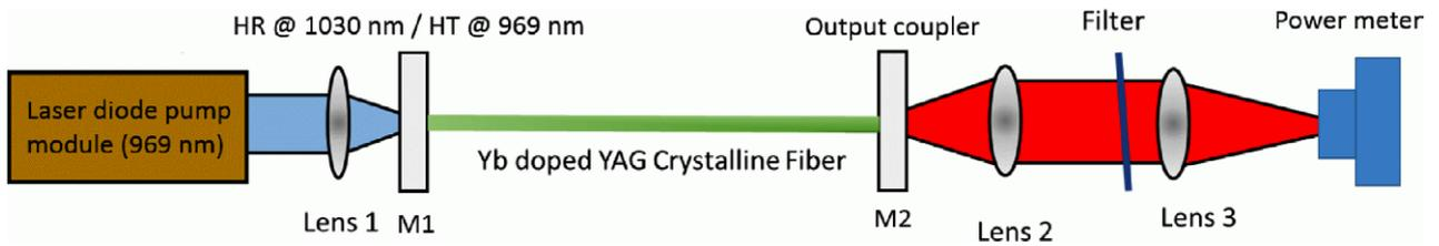
**Figure 1.** Simplified optical layout of the laser experimental setup. A  $\sim 100$  mm long, 1% Yb doped YAG crystalline fibre is free-space-pumped by a laser diode module at  $\sim 969$  nm. Crystalline fibre diameter is  $100 \mu\text{m}$ .
